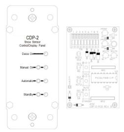
Pressing STANDBY will set the connected snow sensor to ignore snow fall and prohibit automatic the CDP-2 is designed for use either indoors or outdoors with proper protection from the elements.
